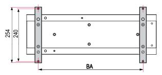
Fig. 9: Fastening set dimensions BA = 300 mm
