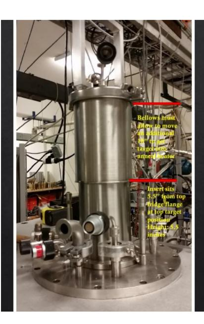
Target insert most bottom out at 5.5" when top cell is in the beamline so that the insert doesn't smash into the nose piece
