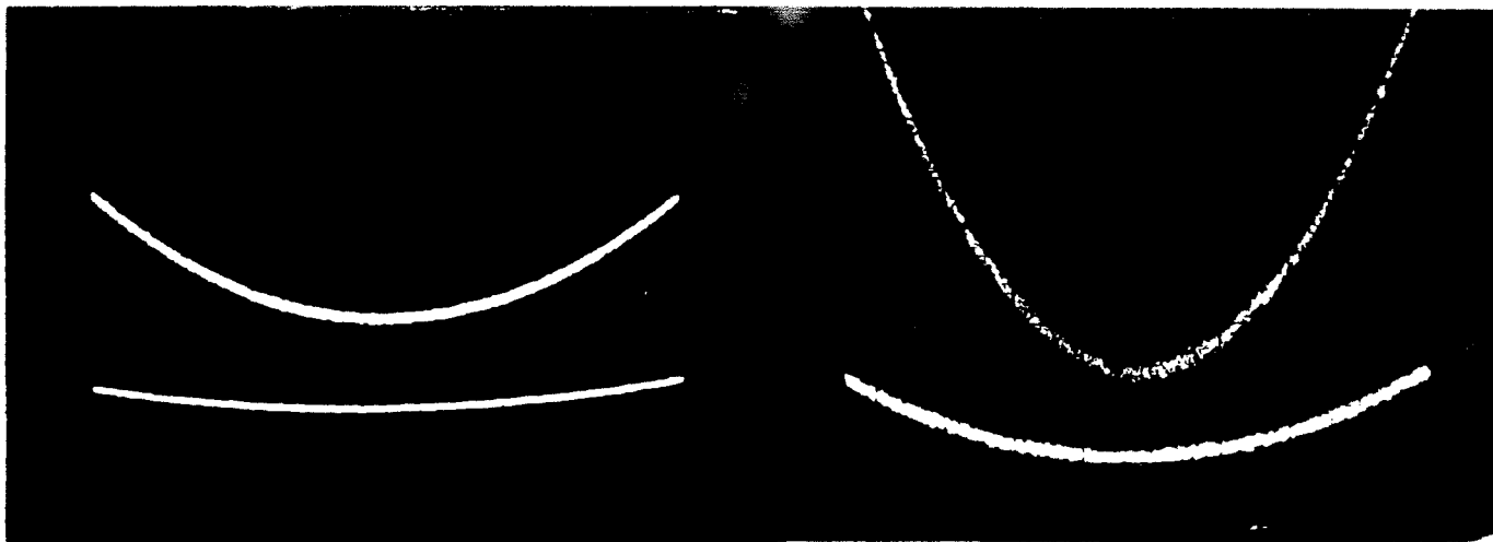
A. BACKGROUND SIGNALS USING TEST CIRCUIT. SCAN = 400 KHZ GAIN X 100 TOP - DIODE CHANNEL BOTTOM - MODULATOR CHANNEL
