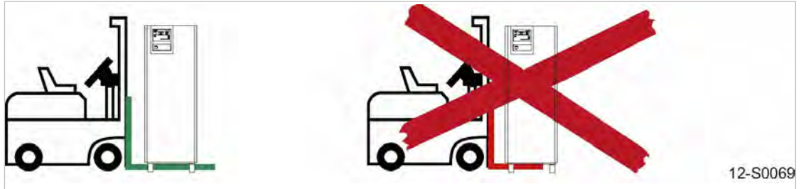
Fig. 34 Transport with a forklift truck
