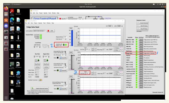
In the above picture, click on Point 1 top open the **Fridge\_Valve** VI, according to Step 12, when the **Heat-Ex Top** resistor goes to 1400 Ohms the interlock becomes red and set the bypass valve at 0.5 turns automatically.
