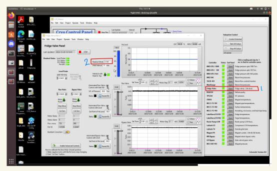
In the above picture, click on point 1 to open the **Fridge valve**. Click on point 2 to put the **Readout Mode** at "**HOLD**" mode.
