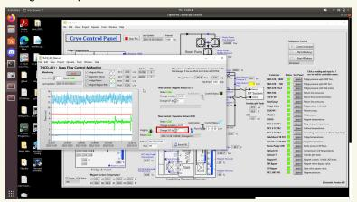
Manually insert 7 at point 1 to set the separator flow at 7 slm.
