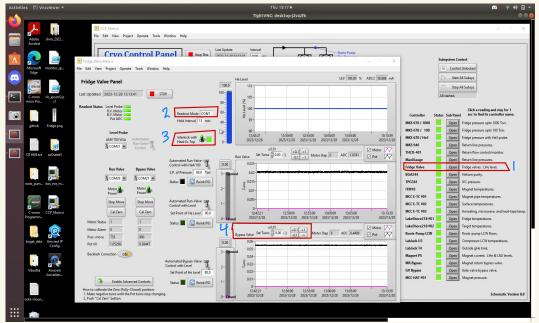
In the above picture, click on point 1 **Fridge Valve** to open the VI to change the readout mode. If the **Readout mode** is not "CONT" mode, put it on "**CONT**" **mode** on point 2. Check the status of **Interlock with Heat-Ex Top**, if it is not on Interlock toggled the button to put it on the **Interlock with Heat-Ex Top** mode.
