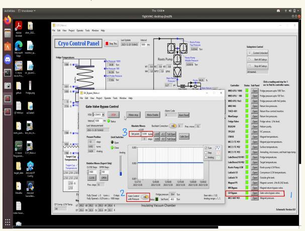
In the above picture , click on the **GV Bypass** on point 1 to open the VI to control **GV Bypass**.
