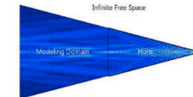
Simulations using RF module in Comsol multiPhysics simulation package
