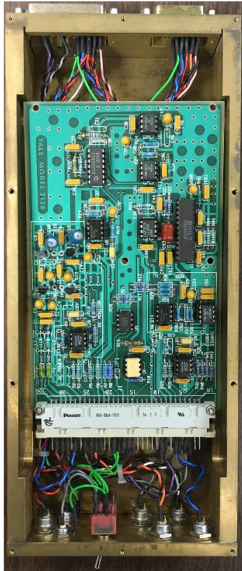
Figure 7.2 (a): Yale card housing with the circuit Figure 7.2 (b): Yale card housing
