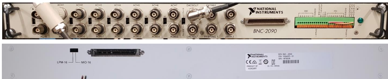
Figure 2.1.1: BNC 2090 (upper: front panel, lower: back panel)
