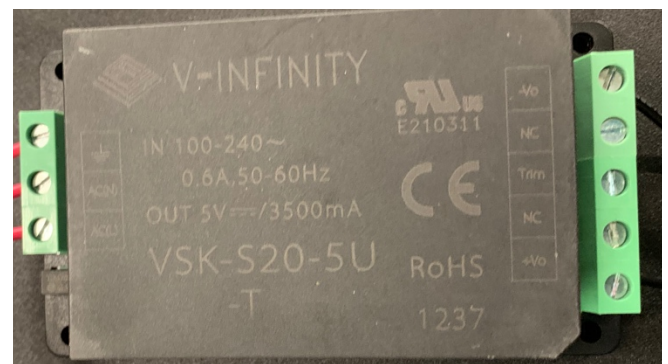
Figure 6.3: DIO box 5V power supply
