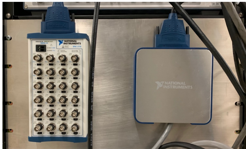
Figure 3.2.1: (left) BNC 2115, (right) SCB-668A
