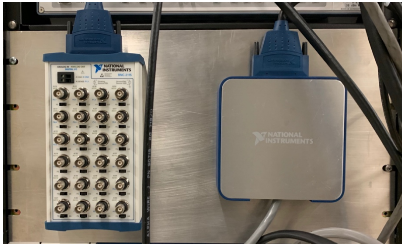
Figure 2.2.1: (left) BNC 2115, (right) SCB-668A
