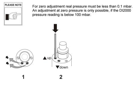
The DU2000 / DU2001 can be used in combination with display units of the DISPLAY or CENTER series. After the adjustment the pressure reading at the display unit at applied zero pressure should be 0 mbar.
