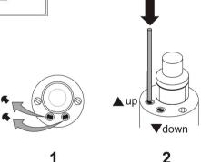
The output signal at zero pressure should equal 4.000 mA (DI2000 / DI2001) or 2,000 V (DU2000 / DU2001).
