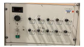
Figure 6: 10-channels shim power supply from Oxford Instrument.
