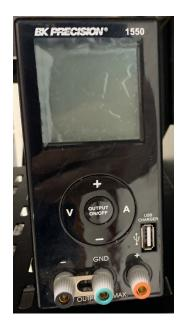
Figure 9: BK Precision 1550 power supply
