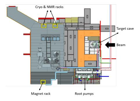
Figure 1: Top view of the cryo platform showing the location of the magnet rack, NMR rack, cryo or target (slow control) rack, root pumps and target cave.
