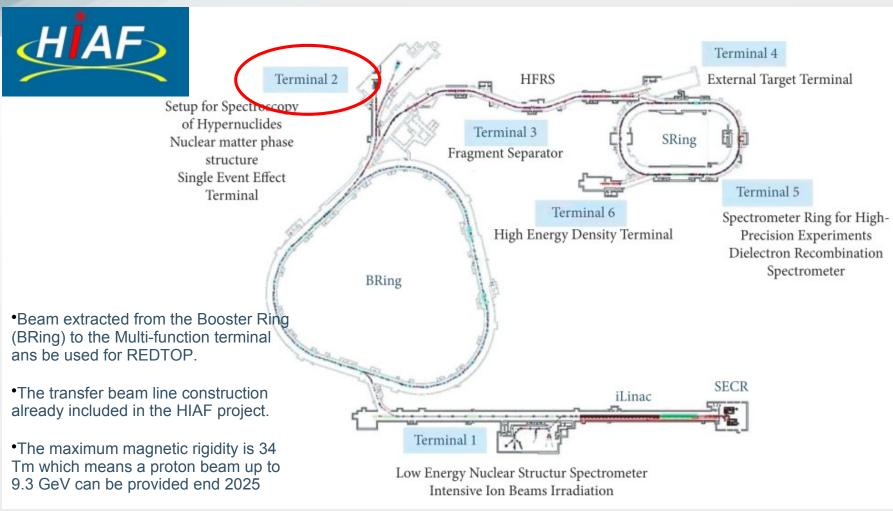
Beam intensity: 0.5 ~1.0x10<sup>13</sup> ppp (1~5\*1x10<sup>13</sup> pps) in Terminal 2 . 10<sup>(18-19)</sup> POT/yr Energy from 2.0 to 9 GeV around 2028 – 2030
