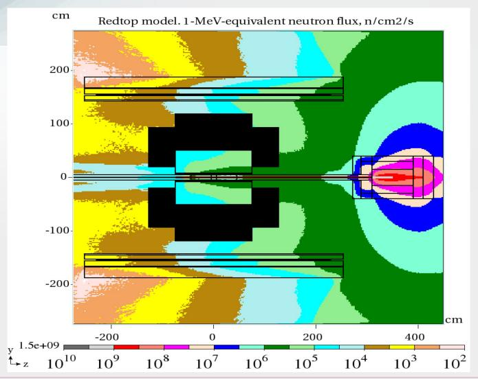
Beam dump:  $dia-30 \times 80 \text{ cm } Al + 15 \text{ cm } HDPE +5\% B + 10 \text{ cm } Barite$
