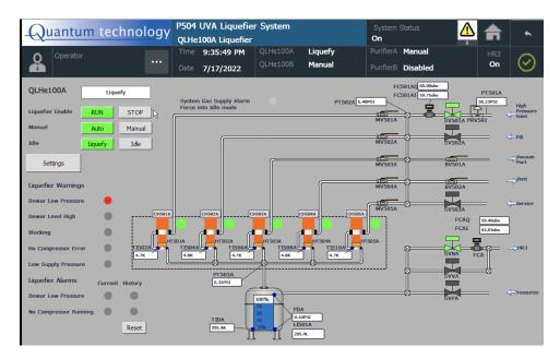
Another possibility of having a "Blockage" at ~4K would appear because HR3 compressor doesn't run. Solution:
