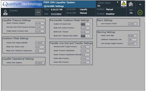
When this is happening, you will see that the cold-heads heaters will turn ON and OFF automatically to regulate the pressure to move towards the "Set point".
