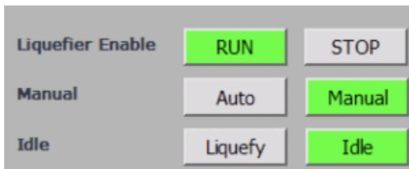
2. Navigate to the liquefier page on the HMI screen.
